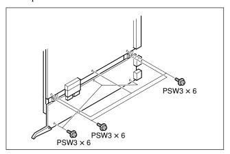
4. Install the MX board. (Refer to this section "HKS-5820M/5830M/5830SD".)
